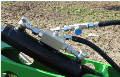
Valve for response speed control of hydraulics
