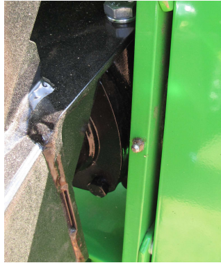
Grease cups of V-belt gearing in suspension box wall Lubrication every 50 running hrs
