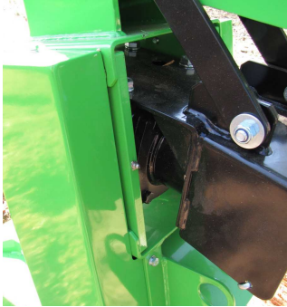
Grease cups of V-belt gearing in suspension box wall Lubrication every 50 running hrs
