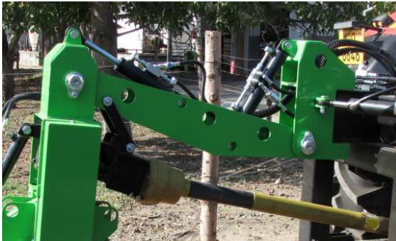
Grease cups of cutting head suspension Lubrication every 50 running hrs
