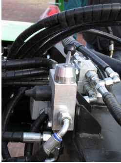
Valve for initial adjustment of oil flow
