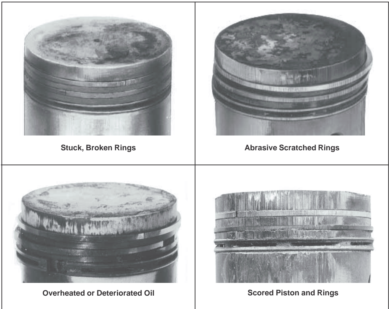
Figure 9-8. Common Types of Piston and Ring Damage.
