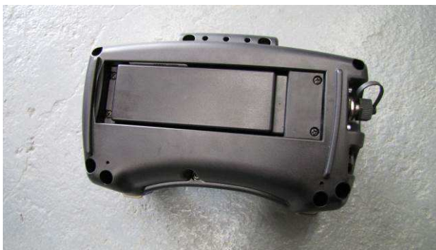
Fig 57 – Remote control box battery
