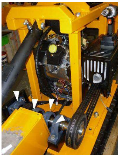
Cutter arm grease points on drive layshaft – covered.
