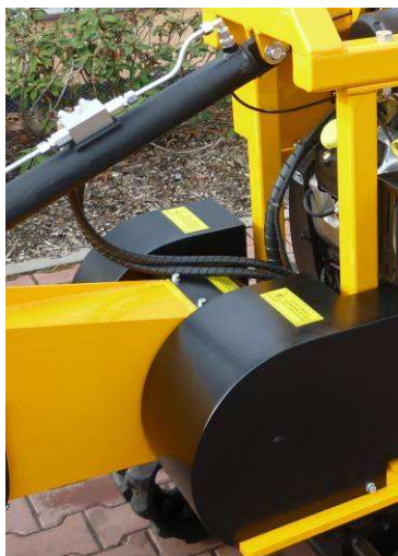
Cutter arm grease points on drive layshaft – covered.
