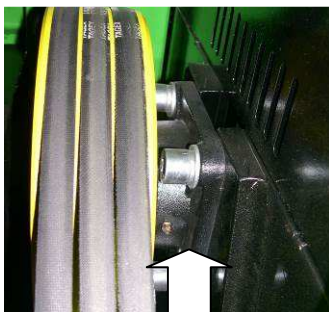
Grease cup of chipping wheel Lubrication every 40 running hrs (weekly)
