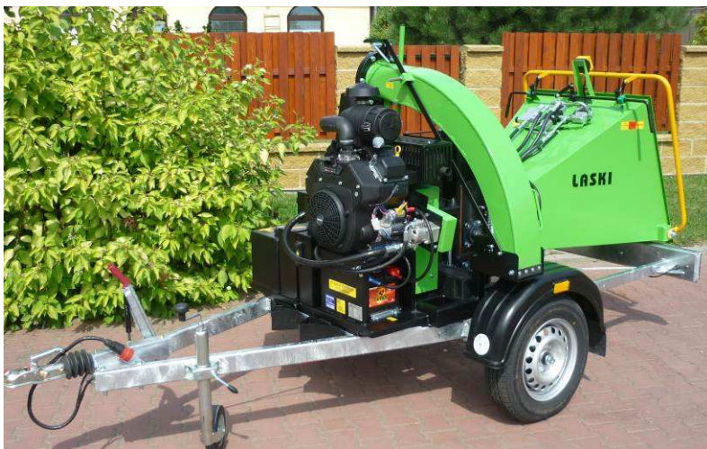
Chipper ready for coupling before transport Discharge duct folded down
