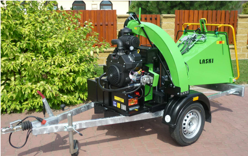
Chipper ready for transport Discharge duct folded down
