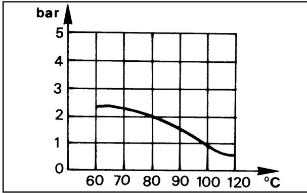
Oil pressure curve at idling speed
