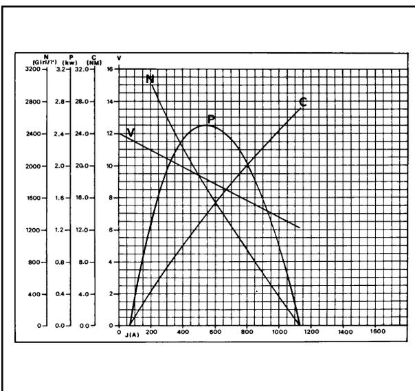
**Characteristic curves for starting motor type Bosch DW (R), 12 V, 1.7 kW**
