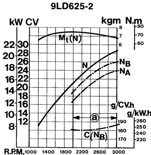
N (DIN 70020)Automotive rating, intermittent operation with variable speed and variable load.
