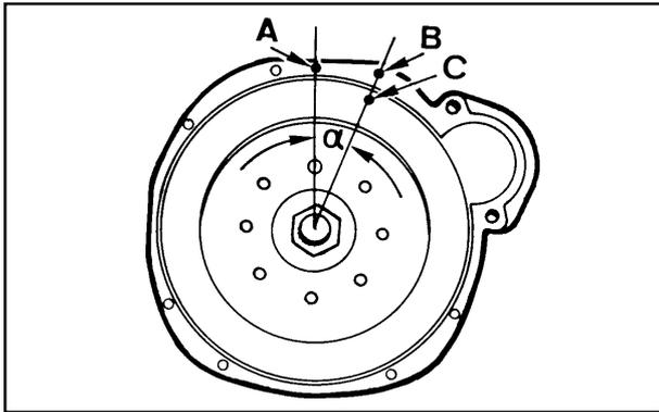
**Injection timing reference marks on crankcase and flywheel**
