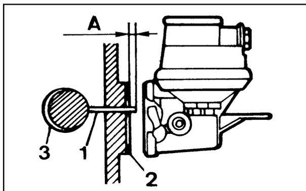
**Fuel feeding pump drive rod protrusion**
