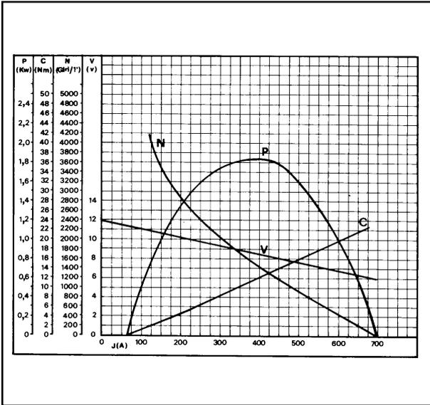
**Characteristic curves for starting motor type Bosch GF -12 V, class 1.5**
