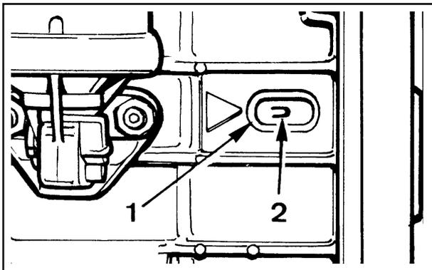
**Check window for injection timing reference mark**
